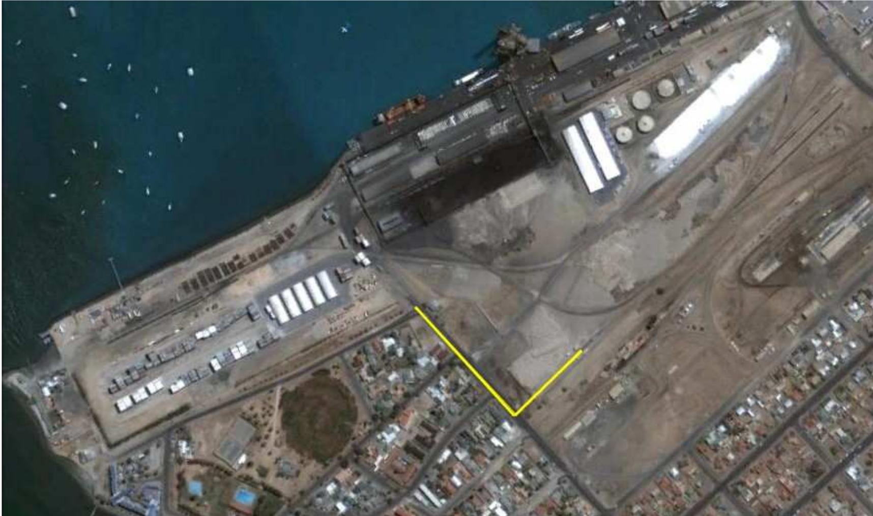
Figure 8.2: Suggested location for a noise barrier wall. Its engineering detail shall be determined when the internal road design is complete.
