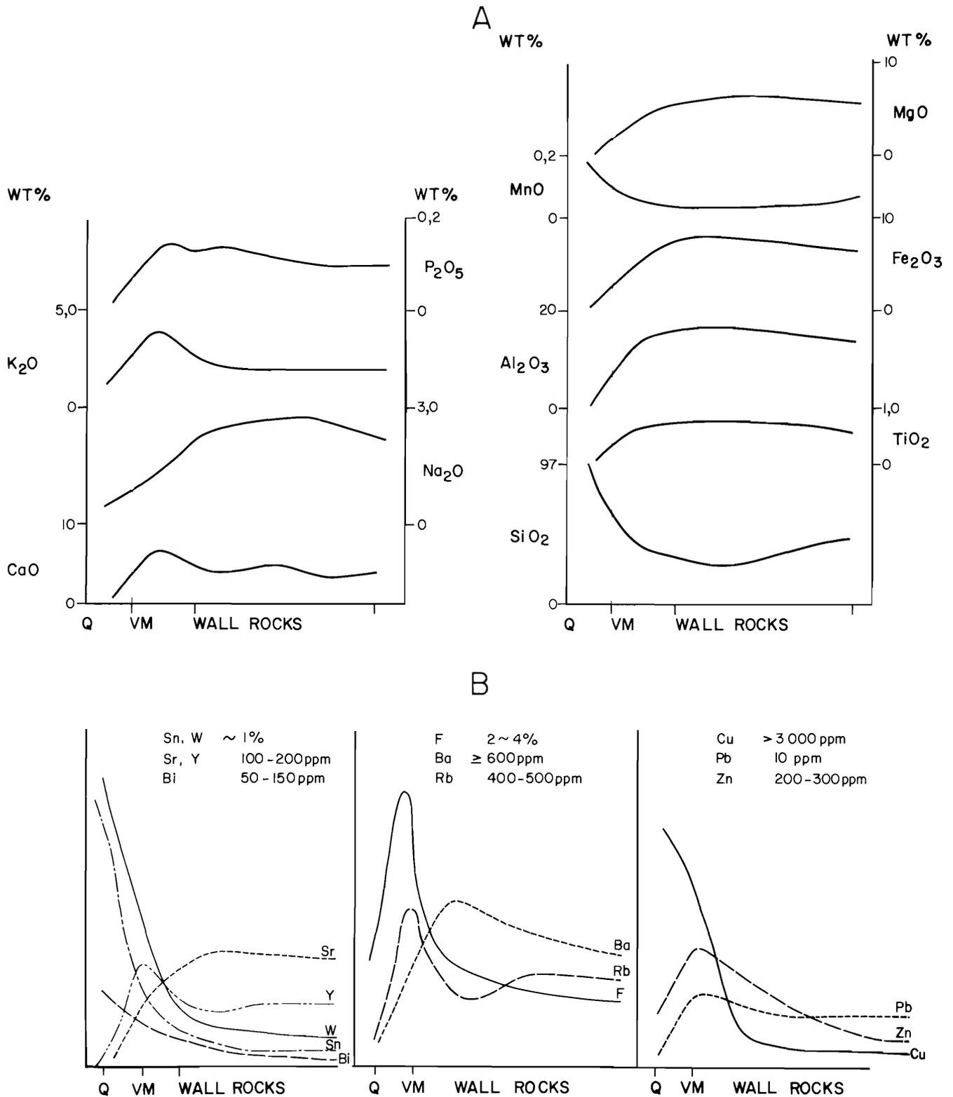
**Figure 11** Diagrammatic summary of (A) major-element, and (B) trace element distribution trends around mineralized veins, based on averages of 3 sampling traverses in Area 1 (greisen stage). Element concentrations in diagram (B) indicate approximate peak values for each element. Q = quartz vein ; VM = vein margin.
