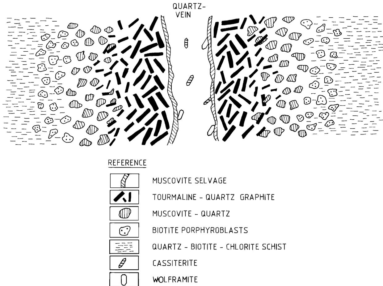
**Figure 7** Diagrammatic representation of the alteration of quartz-biotite schist adjacent to a mineralized quartz vein.
