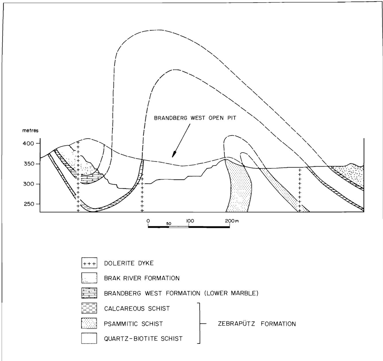
**Figure 4** East-west cross-section across Brandberg West open pit. Modified after Townshend (1985).
