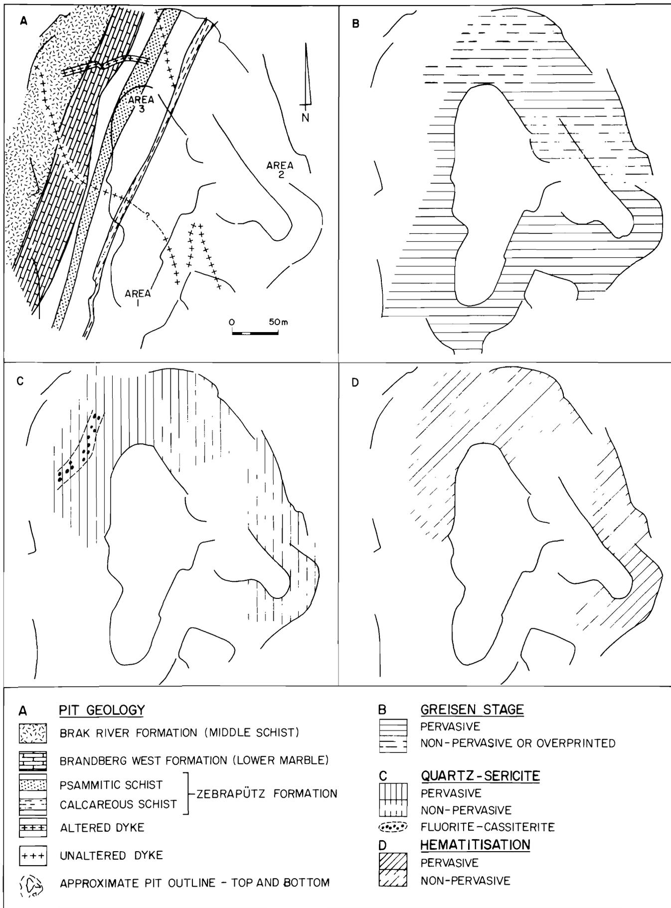
Figure 5 Sketches of the Brandberg West open pit showing geology (A), and patterns of surface alteration (B, C, and D). Modified after Elliott (1985).
