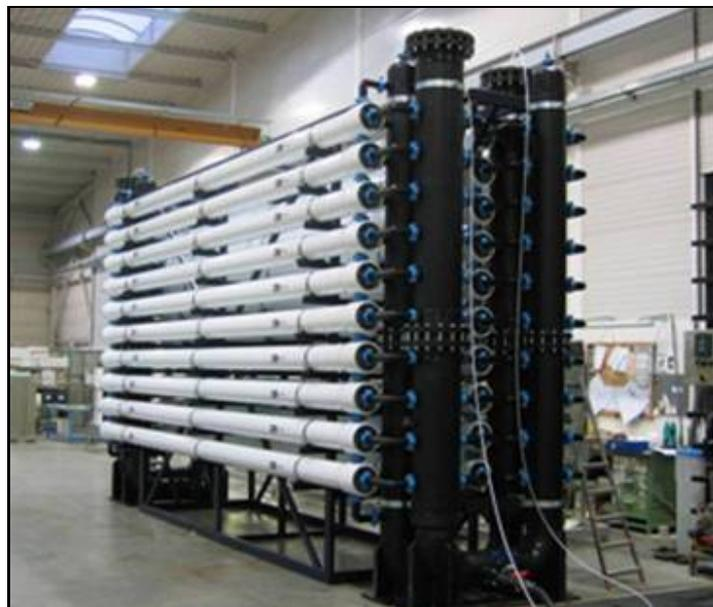
Figure 4 – NORIT Seaguard Ultrafiltration Skid
