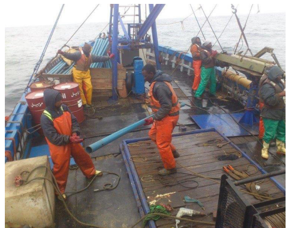
Figure 2: Third generation gravity corer in use.
