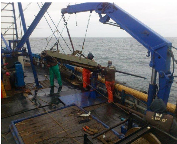
Figure 2: Third generation gravity corer in use.
